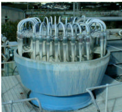
Figure 1: Unit containing multiple 50 mm diameter hydrocyclone separators treating china clay
